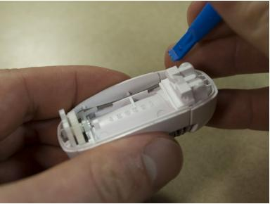
Use Opening Tool to fully depress Tension Clip in place.
