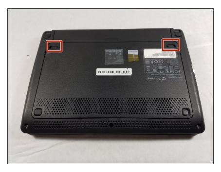
Pull the two marked tabs towards the outside of the computer to unlock them.
