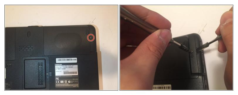
Remove the 5.8mm Phillip's #0 screw with Phillip's #0 screwdriver while prying plastic covering up with metal spudger.
