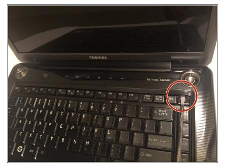
Use the metal spudger to pry out the right portion of the locking piece just above the DEL key.
