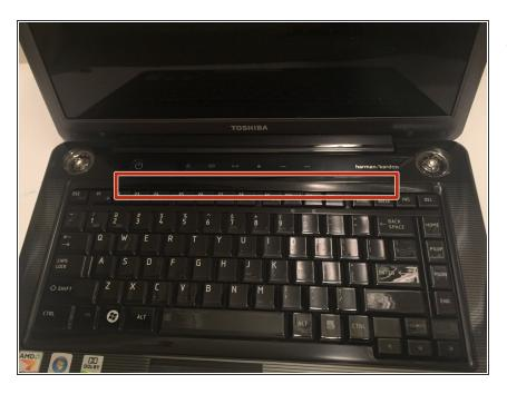
• The keyboard is held in by a locking strip between the screen and the keyboard.
