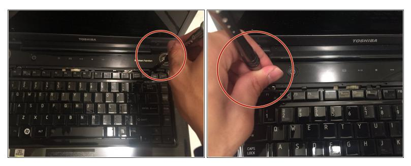
Use the Phillip's #0 screwdriver to take out the two 5.8 mm Phillip's #0 screws from the top right and left corners of the keyboard.
