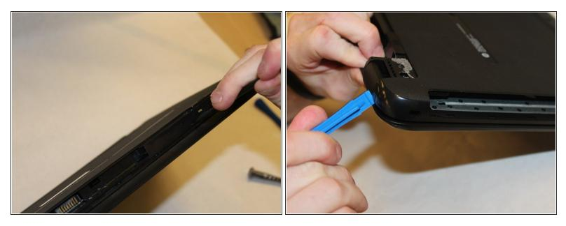
• Use the spudger to press the tabs in the back of the computer. Carefully remove the back of the laptop by prying around the sides using the plastic opening tool.
