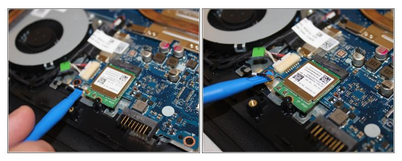
• Using the spudger, carefully pry the wire connecting the wireless card to the motherboard off of it.
