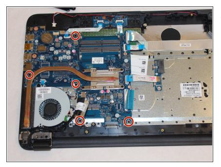
Unscrew the five screws securing the motherboards.
