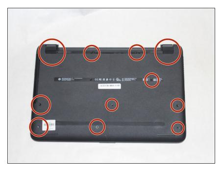
Remove the 11 screws holding the body of the laptop together with a size #00 Phillips screwdriver.
