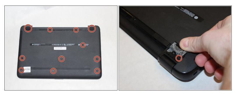
Remove the highlighted screws holding the body of the laptop together with a size #00 Phillips screwdriver.
