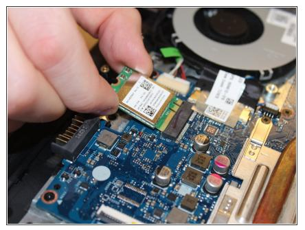
• carefully pull the card of its slot.
