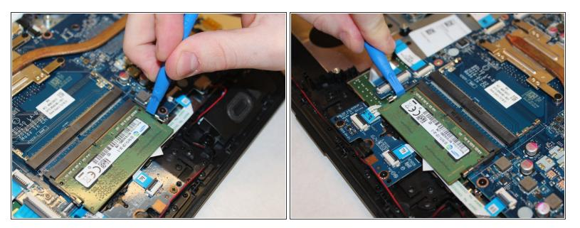
• Undo the clips holding the RAM in place using the plastic opening tool.
