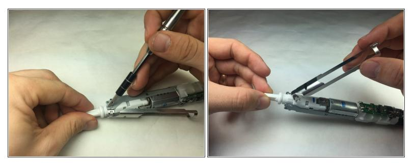
• Use flat head screwdriver to remove power button pressure plate.
