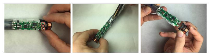
• Desolder the coil wire from the motherboard.
