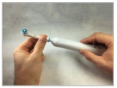
• Remove the brush head by pulling the top away from the base.
