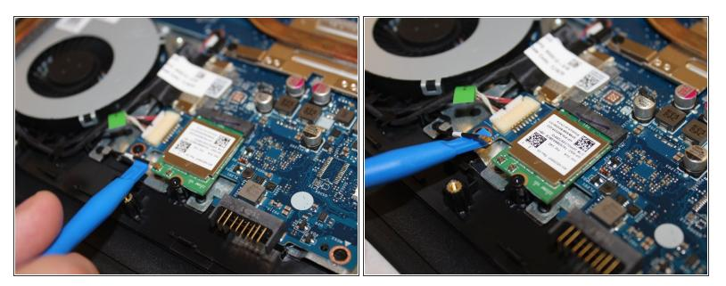
• Using the spudger, carefully pry the wire connecting the wireless card to the motherboard off of it.
