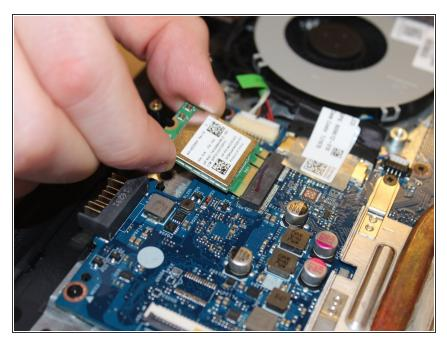
• carefully pull the card of its slot.
