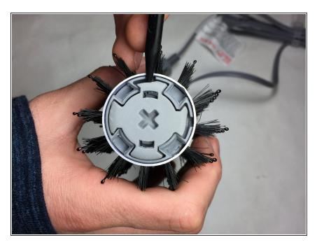
Using the spudger, pry open the sides of the inner cover.
