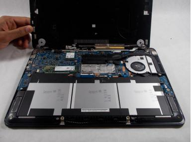
Carefully remove the backplate using the plastic opening tool.
