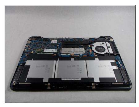
Locate the battery near the bottom.
