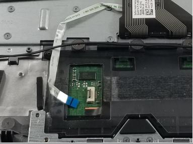
• Lift the flap on the wire connecting the motherboard and remove the connector.
