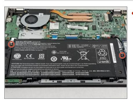
Unscrew the two 5mm battery screws using the Phillips #0 screwdriver.
