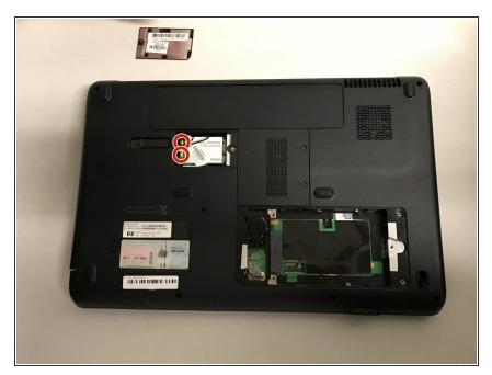
Unhook the two wires attached to the WiFi card.
