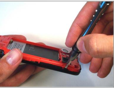
Rotate the phone 180 degrees and loosen the three clips on the side by the speaker. Note that the middle clip on this side is smaller than the others.
