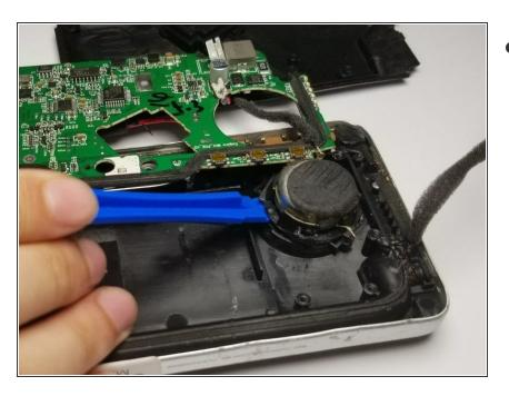
Remove the speaker by using the plastic opening tool. Apply a gentle upward force to remove it.
