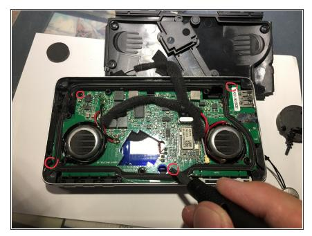
Pull out the motherboard by removing 4 screws around the perimeter of the motherboard. Keep in mind the wires still attached to the speakers, so pull gently.
