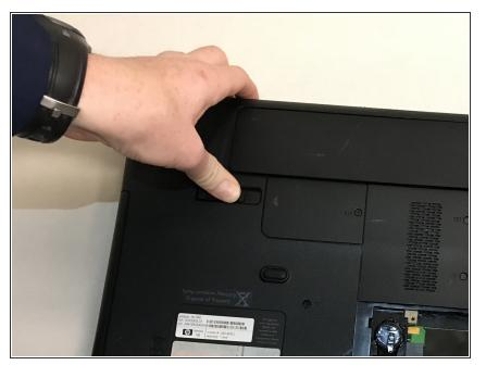
In the top left corner, there is a lever that has a small picture of a battery on it. Slide the lever to the left.
