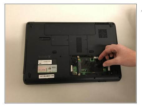
Once the screws attached to the hard drive are removed, you will be able to take the hard drive out of the compartment.
