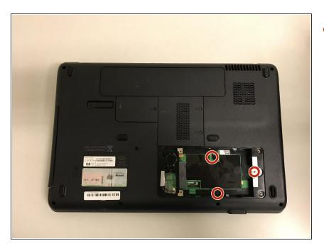
After the panel has been removed, use the screwdriver to remove the three 3mm Phillips #0 screws attached to the hard drive.
