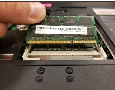
Grab onto the module and pull away in a straight direction.
