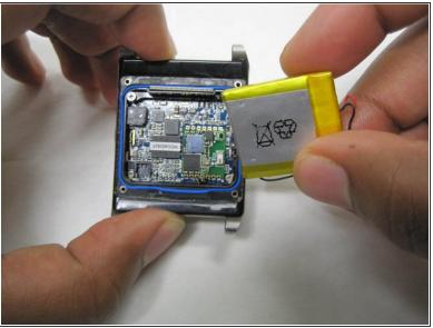
Use the flat end of the spudger to carefully lift the battery until adhesive seal is broken.
