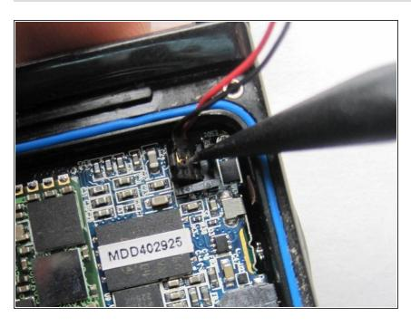
Use the pointy edge of the spudger tool to detach battery leads from the circuit board.
