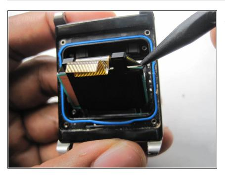
Use spudger tool to remove the LED screen from the watch case.
