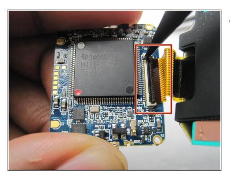
Use spudger tool to lift the clasp of LED connector strip and remove from watch case.
