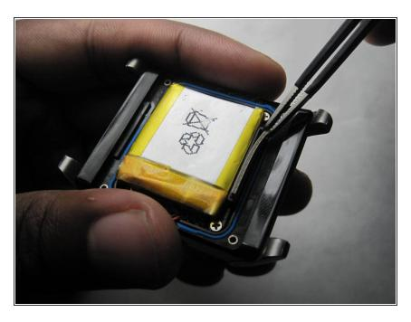
Use tweezers to remove elastomeric, or zebra, connector.
