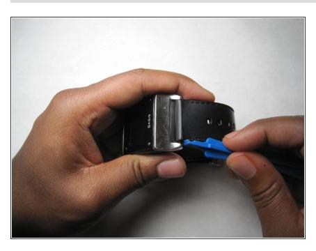
Wedge a plastic opening tool between band contacts.
