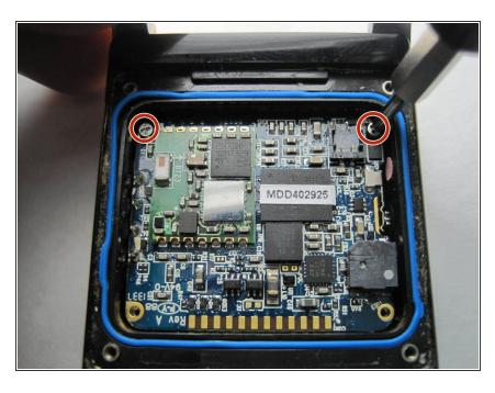
Use PH000 tool to remove two 4mm screws.
