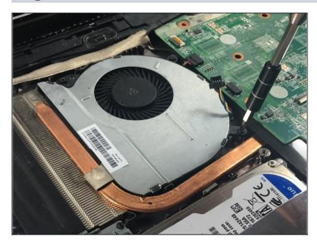
Unscrew the three 6.0 mm screws on each corner securing the cooling fan with a Phillips #0 screwdriver.
