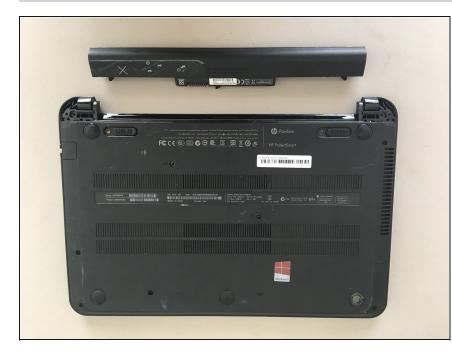
Remove the battery by sliding it upwards and away from the computer.
