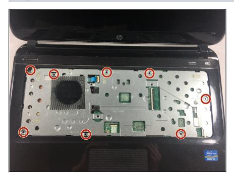
Remove the eight 6.0 mm screws located under the keyboard with your Philips #0 screwdriver.
