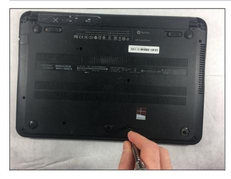
• Unscrew the ten 6.0 mm Philips head screws on the base of the device with a Phillips #0 head screwdriver.
