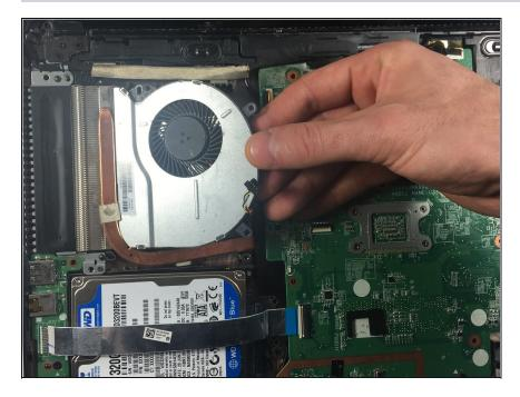
Remove the cooling fan by lifting upwards and pulling to the right.
