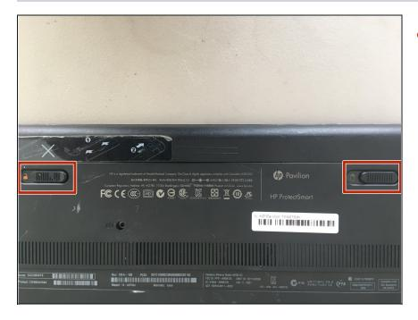
Slide the left release tab toward the center of the computer to the unlock position. Next slid the right tab toward the center of the computer and hold it there while completing step 4.
