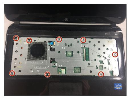
Remove the eight 6.0 mm screws located under the keyboard with your Philips #0 screwdriver.
