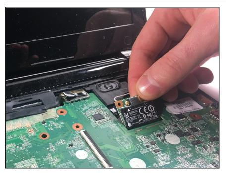
Once you have removed the screws and wires on the network card lift it up and away from the motherboard.
