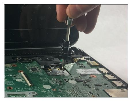
Remove the two 4.0 mm long screws on the corners of the wireless card the using a Philips #0 screwdriver.
