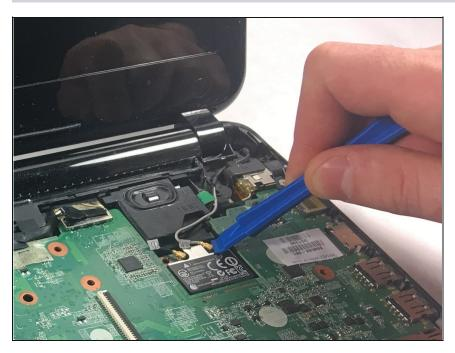
Remove the black and white wires attached to the wireless card by using your blue opening tool and prying upward.
