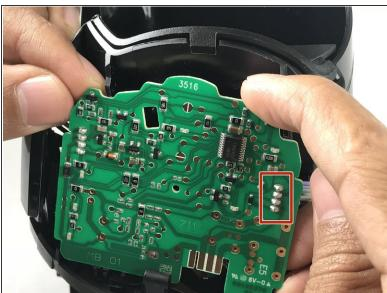
Remove solder from wire harness leading to the charging base motor.
