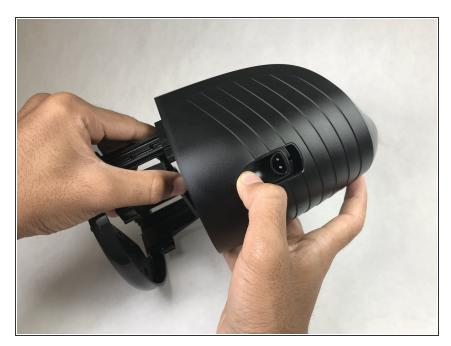
Press inward on the side charging port while pulling cover from the base to separate.
