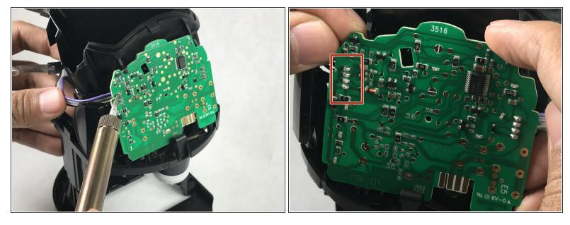
Remove solder from circuit board and remove charging harness.
