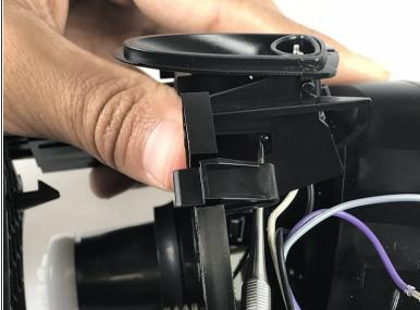
Remove side charging port by prying tabs outward and rotating port upward.
