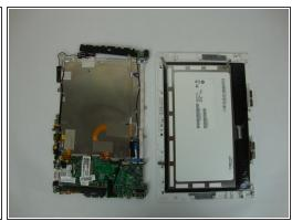
Very carefully lift the circuit board in order to keep everything attached. Be careful with any cables that may still be connected.
