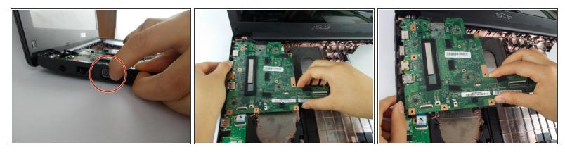
Push on the VGA port and wiggle the motherboard out.
