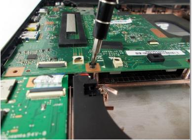
Remove the Phillips #0 screws securing the motherboard to laptop.
