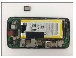
Using the tweezers, slide them under the speaker and pull the speaker out.
