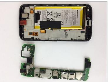
• Using the tweezers pull up on the three corners of the motherboard until it comes out.
