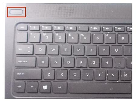
Turn power off using the power button located in the top left corner of the keyboard. Press and hold the power button for 3 seconds until it turns off.
