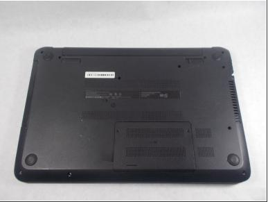
• Close the laptop and flip it over so that the HP cover logo is on the underside of the laptop.
