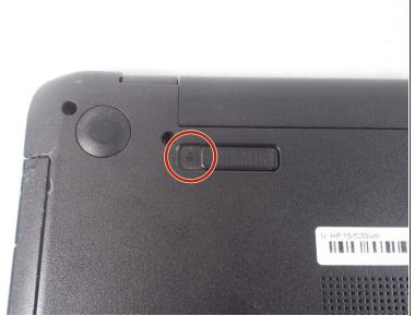
Slide the left switch to the right so that the icon of a locked padlock is no longer visible and the icon
