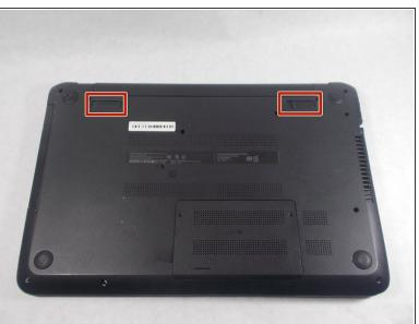
Locate the battery and the two switches that release the battery when they are unlocked.
