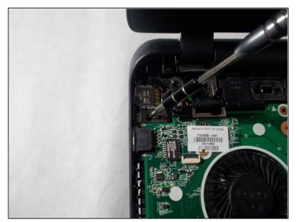
After removing the battery and the palm rest, remove the two 7 mm PH1 Phillips head screws holding in the small metal power jack holder.
