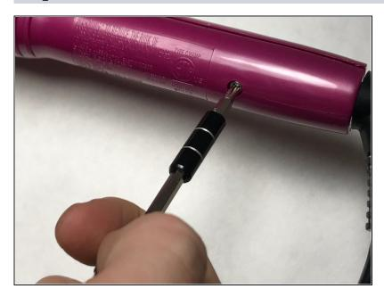
• Remove the Philips #1 22 mm screws.
