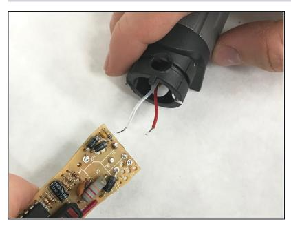
Once both wires are desoldered the motherboard can be removed.
