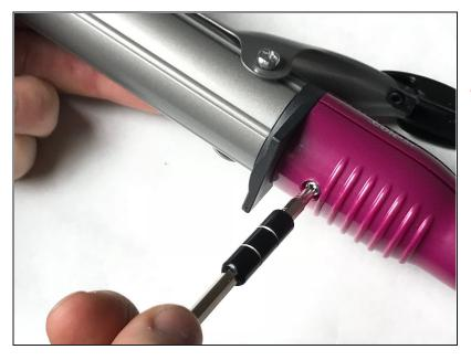
• Remove the Philips #1 28 mm.
