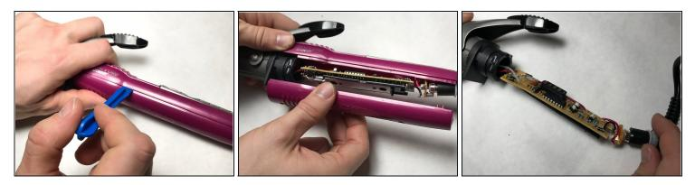
• Pry off the housing using a plastic spudger.
