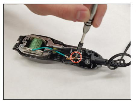
Remove one 7.5 mm JIS #1 screw connecting the power cord to the switch base.
