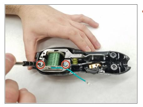
Remove two 23.0 mm JIS #1 screws attaching motor base to device body.
