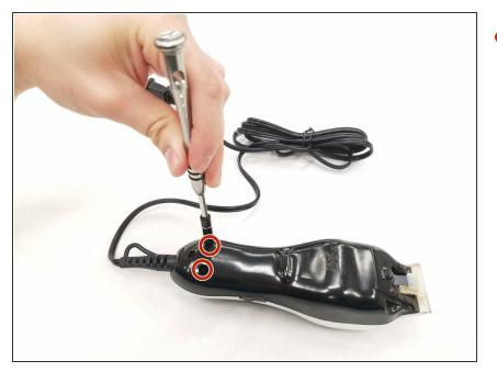
Remove the two 12.0 mm JIS #1 screws on the back of the device body.
