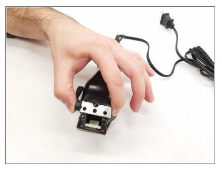
• Lift the base of blade assembly straight up off of the body.
