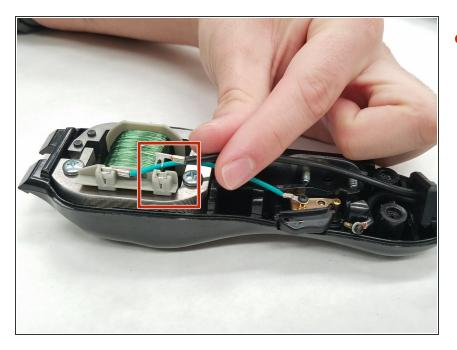
Lift power cord tab (black wire) from slot on motor base.
