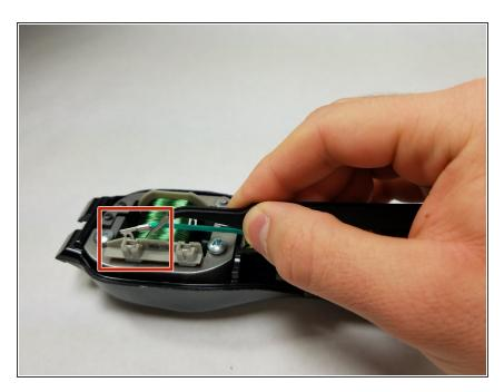
• Lift switch tab (teal wire) from slot on motor base.
