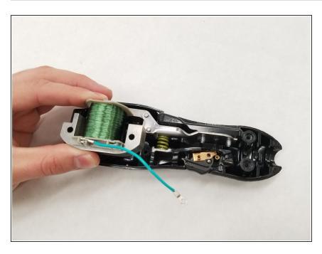
• Lift motor base straight up from device body to remove.
