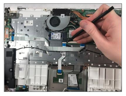
Use the spudger tool to unhook the locks on both sides of the end of the white ribbon. Pull the ribbon outward away from the motherboard.
