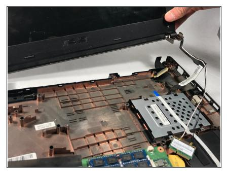
• Once both sides of the laptop are unscrewed, gently pull the upper half of the laptop off of the bottom half.
