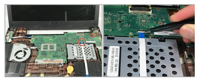
• Unlatch the data cable by using tweezers to lift the white tab and release the cable.
