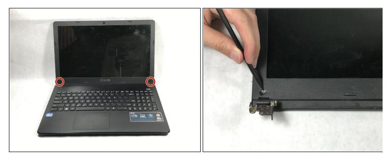
• Use the black plastic spudger to pry off the black squares on the bottom of the laptop screen, this reveals two screws.
