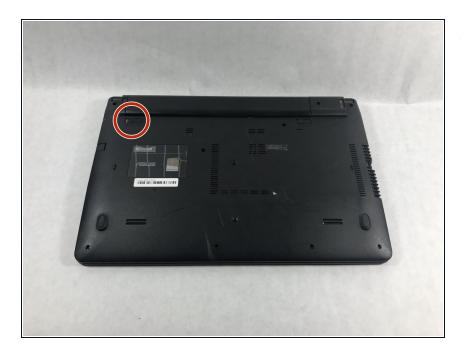
• To unlock the left tab, make sure the tab on the left has red showing.
