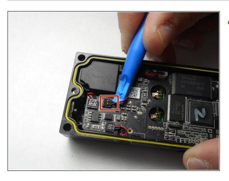
Remove this wire connection by gently prying it off with a plastic pry tool.
