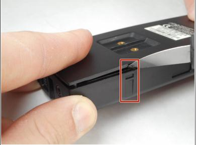
Using a plastic pry tool, go along the edge of the device prying the device apart. While doing this, focus on the four clips, two of which are on either side of the device.
