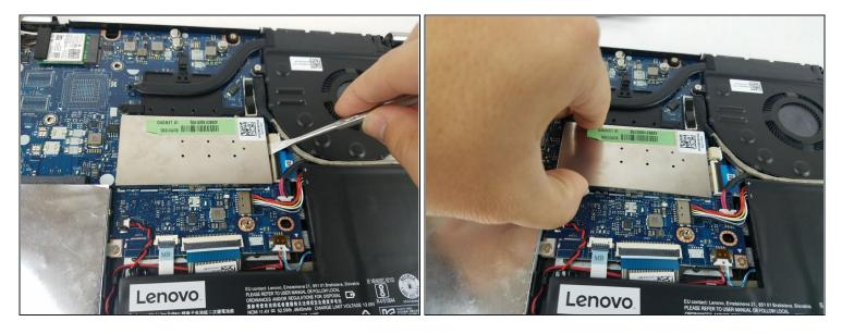
A RAM cards can be damaged from exposure to a static charge through contact with the hand or other body parts. Though the damage of one discharge is not severe, multiple exposures can cause your RAM to fail.
