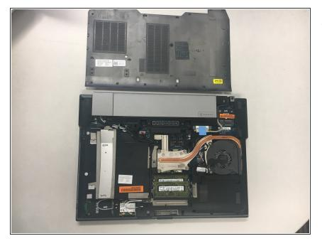
• Remove the back cover by sliding it downwards.
