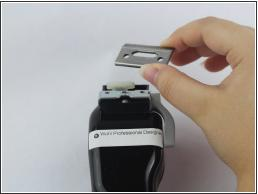
• Unscrew the 6.2 mm Phillip head screw using a Phillip's #1 screwdriver and remove the blade.
