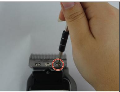
Unscrew the two 3.8 mm Phillip head screws located on the blade using a Phillip's #0 screwdriver.
