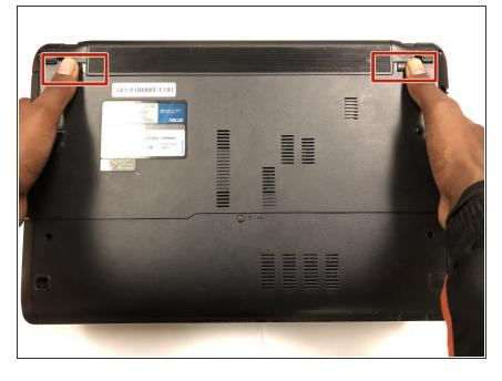
Push the two tabs located at both corners of the laptop, outwards using both thumbs.
