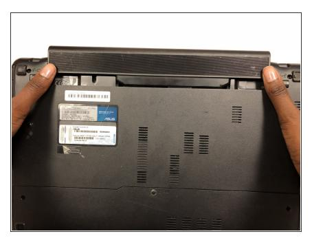
Push the battery upwards as shown in the image for the battery to detach.
