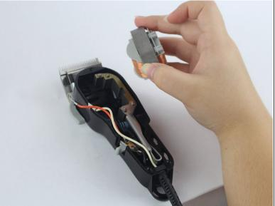
Gently remove the motor from the device.
