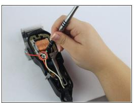
• Unscrew the two 20.5 mm Phillip head screw located on the motor using a Phillip's #1 screwdriver.
