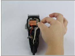
Remove the wires connected to the motor by firmly grasping both sides of a wire and wiggling until it is released.
