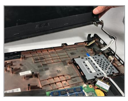
Once both sides of the laptop are unscrewed, gently pull the upper half of the laptop off of the bottom half.
