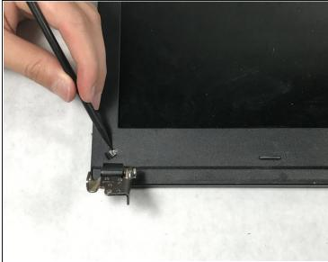
• Use the black plastic spudger to pry off the black squares on the bottom of the laptop screen, this reveals two screws.
