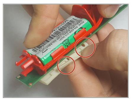
Remove the white circuit board cover as shown. This cover will require you to pry off the piece from the groves.
