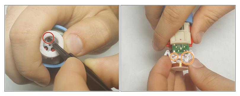
Remove the internal electronic mechanism from the housing by prying the red clips shown in the figure. This removes the charging port.
