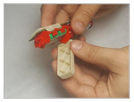
• Remove the white battery cover as shown in the figure.
