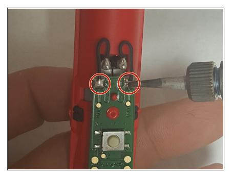
• Desolder the motor from the circuit board at the two locations shown.
