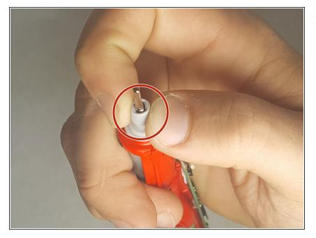
Disassemble the device. Remove the plastic piece over the brush attachment as shown. Object can be removed by hand as shown. No tool is required.
