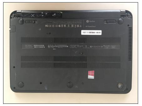
Place the device on your work surface with bottom facing up and the battery located at the top.
