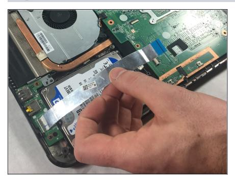
Gently unhook the ribbon cable blocking the hard drive by lifting the locking bar with a plastic opening tool.
