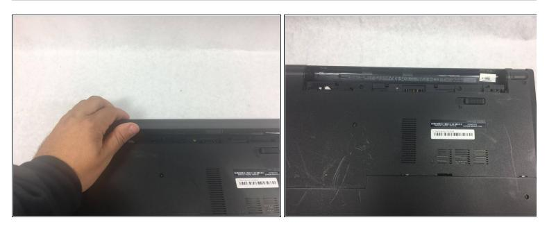
• Rotate the battery up and remove it.
