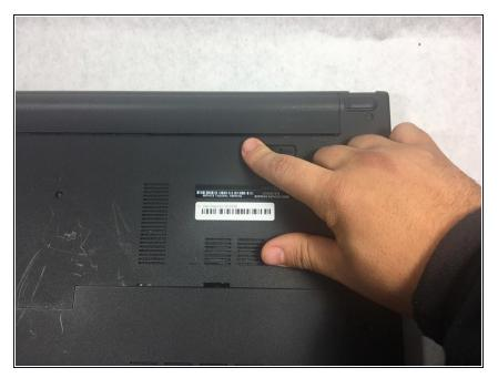
• Slide the battery latch all the way to the left until you hear the click and see the battery prop up.
