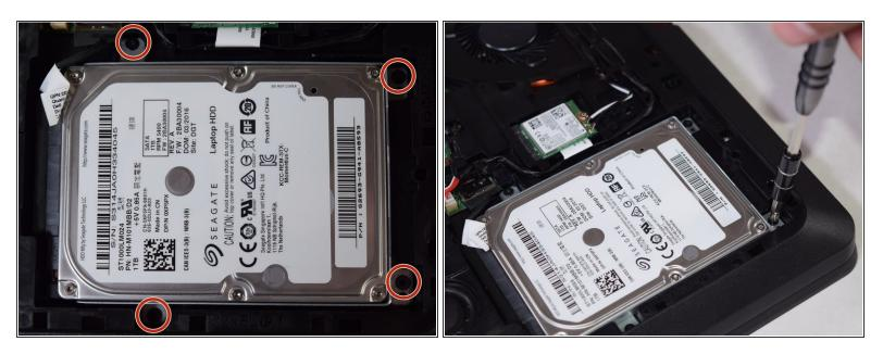
Unscrew the 4 x 2.5mm x 5mm screws, using the Philips #1 screwdriver.
