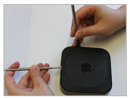
As the Apple TV doesn't have any visible screws or points of entry, the first step is to use a couple of metal spudger to carefully loosen and remove the rubber base/bottom cover from the upper case.
