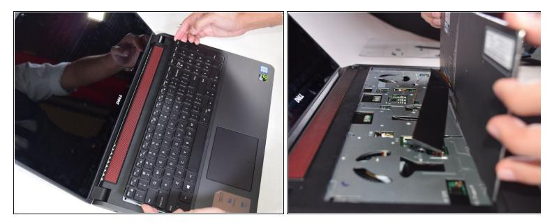
• Now lift the keyboard enough to access the ribbon cables beneath it.
