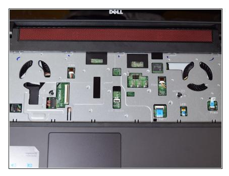
• Now that the keyboard has been fully disconnected from the laptop, lift it off of the device.
