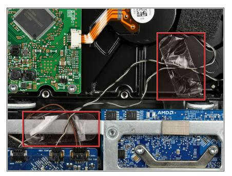
If necessary, remove the pieces of tape securing the hard drive/optical drive thermal sensor cables to your iMac.
