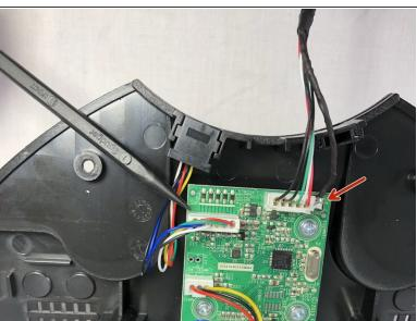
Using a small plastic opening tool, gently pry up the white connector that connects the USB cable to the board.
