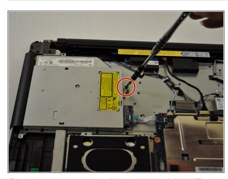
Using #1 Phillips screwdriver remove the 1 (9mmx6mm) screw holding the disk drive in place.
