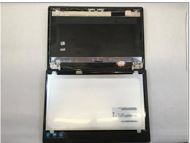
Carefully lay the screen facing down on the keyboard.
