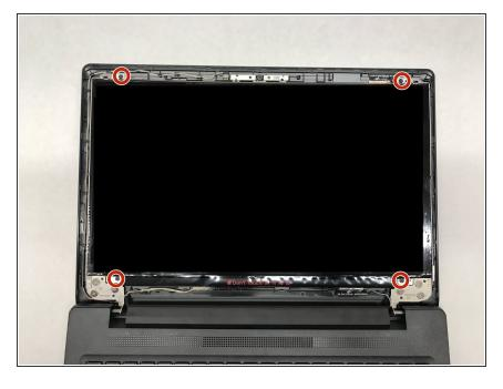
Using the #1 Phillips head screwdriver unscrew the 4 (9mmx6mm) screws holding the screen in place.
