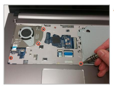
Remove four 7mm Phillips #1 interior screws.
