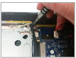
Unscrew the battery from the laptop by removing two 3mm Phillips #1 screws.
