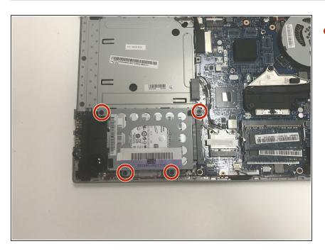
Remove the four 3mm Phillips #1 screws holding in the hard drive.
