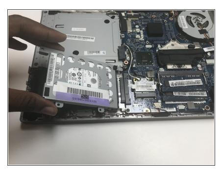
Lift the outermost end of the hard drive and slide it out of the connector to disconnect it from the motherboard.
