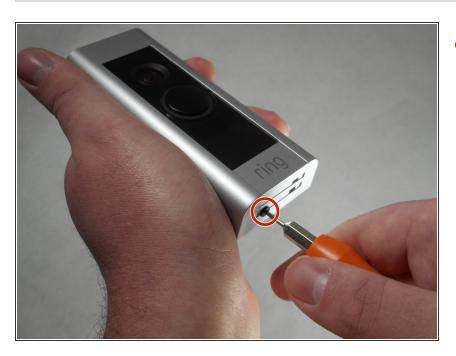
Start by using the star-shaped end of the included Ring screwdriver to take out the 5 mm screw on the bottom of the device.
