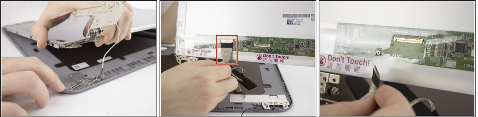
**⚠** Be sure not to damage the display cable when lifting the screen!
